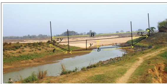
Figure 17: Flood Estimation of the River Area Showing the Trapezoidal Shape
