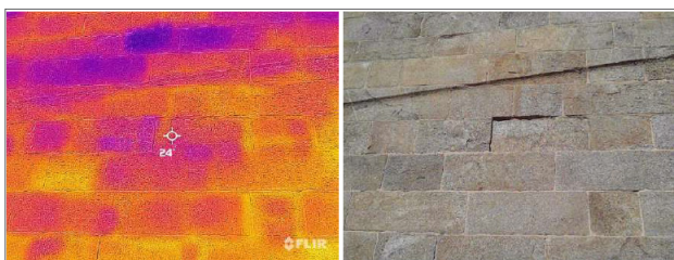
Figure 13: Detailed thermographic analysis of the constituent materials (granite with mortar) of a fragment of the façade of the Torre de Hércules Roman lighthouse. We can see, on the left, the photograph taken by a thermographic camera and, on the right, the same photograph taken by a photographic camera (photographs by the author).
