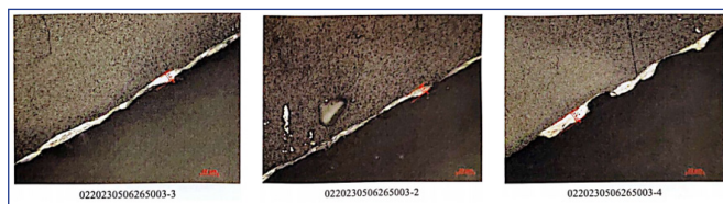
Figure 17: Schematic diagram of experimentally tested remelted layer thicknesses. (The three diagrams from left to right show the thickness of the remelted layer on different surfaces).
