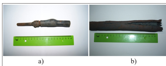
Figure 3: HEC billets at 940°C with intensity of loading under 10GPa
