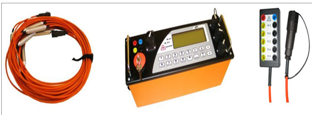
Figure 4: ARES Units ( Equipment Used)
