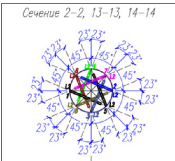
Figure 3: Scheme of injection wells (plan in axes “B” and “M”)
