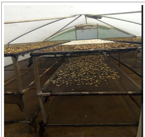
Figure 4: Showing solar drier with pumpkin seeds and bananas drying at the Natural Ways Food Supplement Ltd based in Tetu, Nyeri County.
