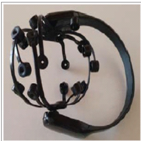
Figure 2: The EMOTIV/EPOCx EEG equipment with 14-channel. The serial number is E2020730
