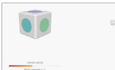
Figure 8: The data obtained by using the EMOTIV / EPOCX EEG equipment with 14-channel and with equipment serial number E2020730. Note: By means of the special software of EEG device it is possible to manipulate the cube on the computer screen just by brain thinking and it is possible to simulate facial movements and facial expressions on the computer screen, as well
